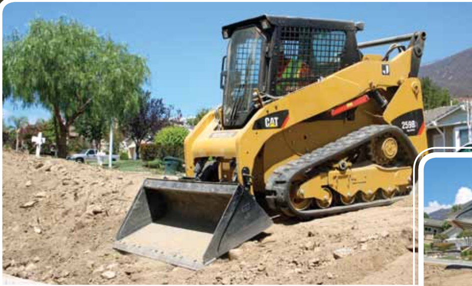
Left & Below: Caterpillar 259B Skidsteer back dragging sloped grade prior to installing jute and fiber webbed erosion control. This versatile machine may also be equipped with an auxiliary auger, trencher, rototiller, landscape rake, and numerous other implements.
