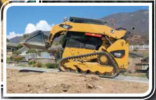
Left & Below: Caterpillar 259B Skidsteer back dragging sloped grade prior to installing jute and fiber webbed erosion control. This versatile machine may also be equipped with an auxiliary auger, trencher, rototiller, landscape rake, and numerous other implements.
